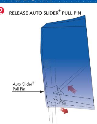
With one hand, slighty push up on the truss near the **Auto Slider® Pull Pin** to relieve pressure.
