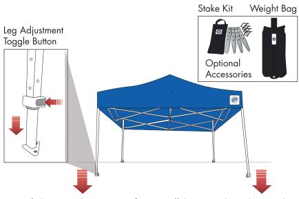
Lift the two adjacent **outer legs** up off the ground simultaneously to about waist height.
