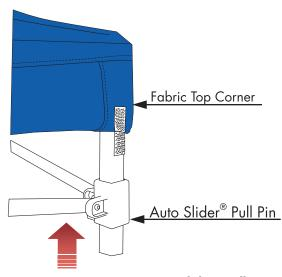
Fold up the fabric top corner to expose the Auto Slider® Pull Pin.
