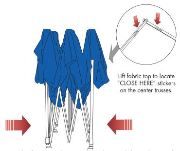
Grasp the frame on the top of the diamond-shaped area of **center trusses** on the opposite sides near the "CLOSE HERE" sticker.
