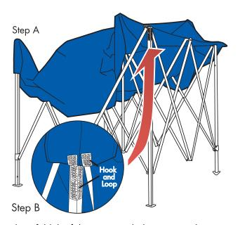
Gently unfold the fabric top, and place it over the semi-opened frame.
