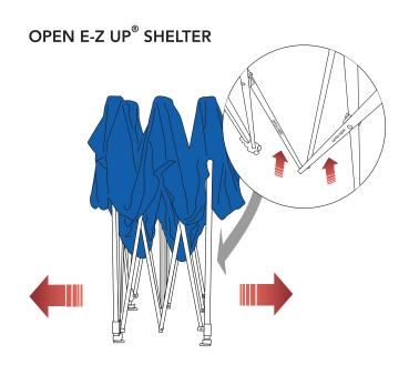
With a partner on the opposite side, grasp the bottom of the diamond-shaped area of **outer trusses** near the "OPEN HERE" sticker (see arrows for OUTER TRUSSES on the diagram on page 7 for approximate location of "OPEN HERE" stickers).
